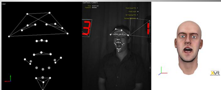
Figure 2. Performance-driven Animation: Facial Template (Left), marker based mocap (Middle), and animation (Right)
